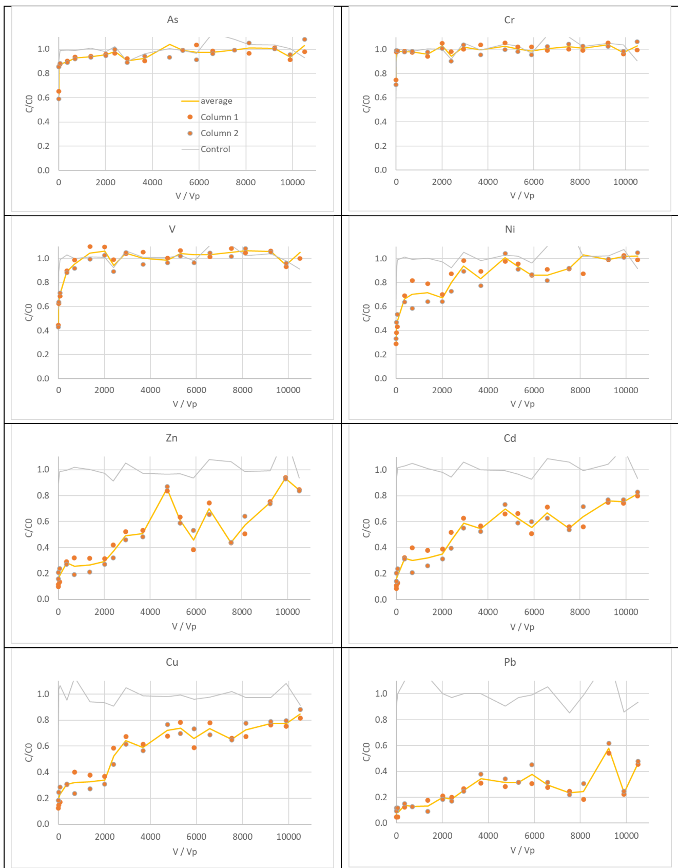
Figure 25 : normalized trace metals breakthrough curves ( C = outflow concentration, C_0 = inflow concentration, V = cumulated volume, V_p = pore volume of the column)
