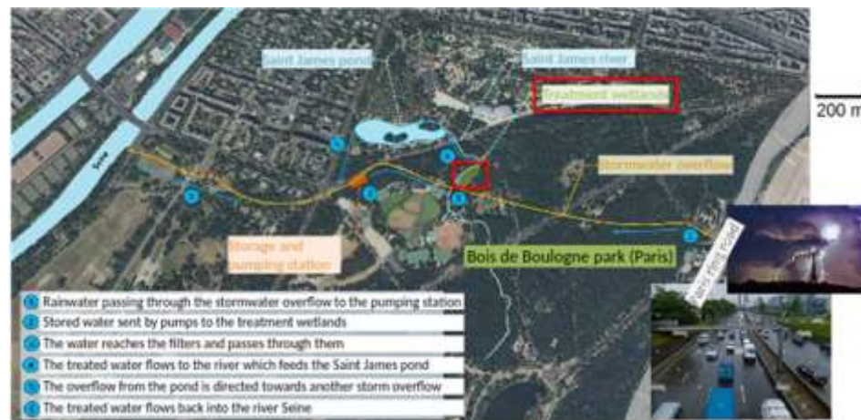
Figure 27. Water flow, from the Paris ring road to the filters and then to the Seine
