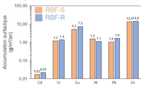
Surface accumulation (g/m<sup>2</sup>/year) of TMs on the scale of RBFs
